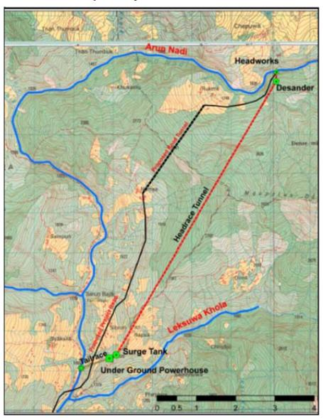
Annex 5. Salient features of the Upper Arun Hydropower Project, as derived from the feasibility study completed in 1991.
